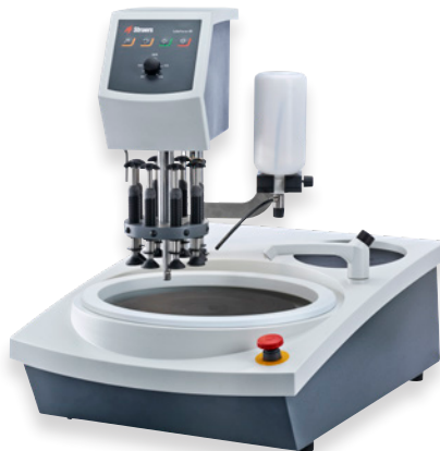
LaboForce-Mi is a semi-automatic specimen mover for the production of thin sections, polished thin sections and polished specimens of mineralogical materials. The force is applied through springs which can be individually adjusted
