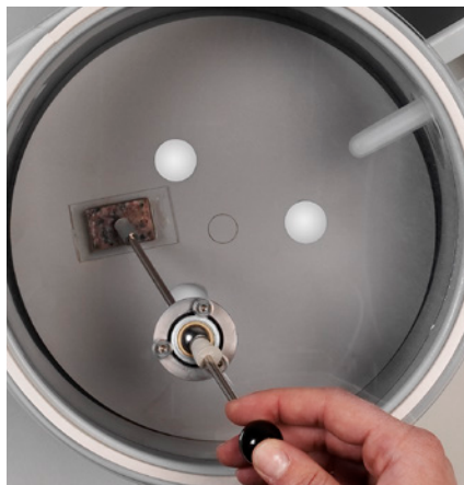
A special lid has to be used when gluing specimens to glass slides with the CitoVac.
