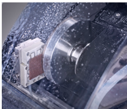
Grinding with cup-wheel on Accutom-100.
