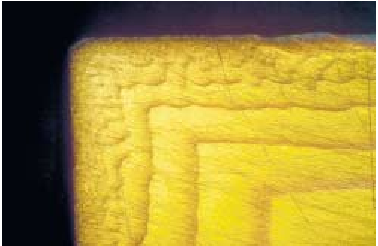
1. Smearing on soft, ductile steel Mag: 15 x, DIC
