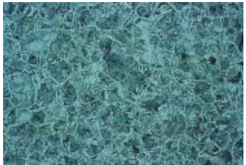
Medium carbon steel, overheated Mag: 200x Etchant: Nital
