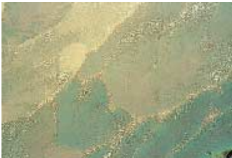
Eutectic copper alloy with 8.4% P Mag: 100x Etchant: Klemm III
