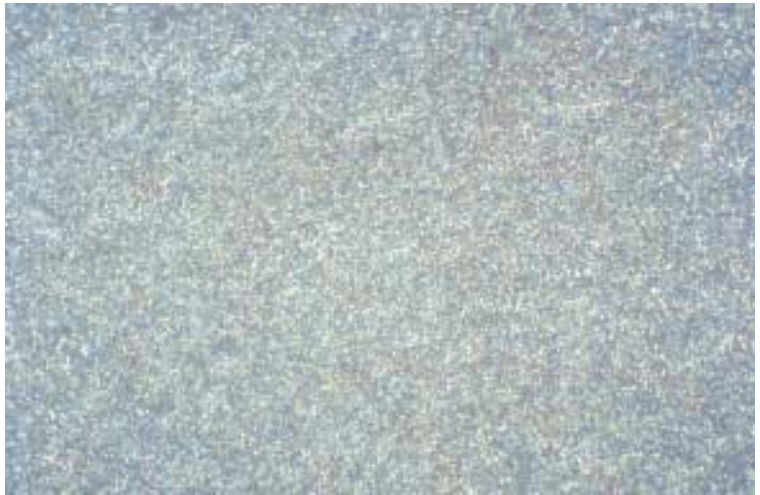
100 Cr 6 Mag: 500x Etchant: Nital
