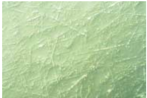
2. Well-defined, sharp deformation lines Mag: 200 x, DIC
