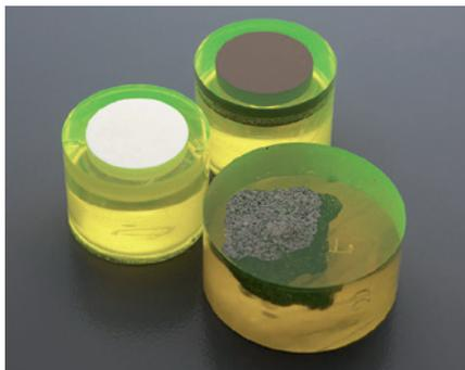
Struers fluorescent dye makes it easy to identify pores and cracks
