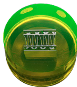
EpoDye, fluorescent dye to be mixed with the resin to allow for easy identification of pores and cracks when examining the specimen in fluorescent light.
