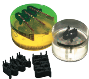
The MultiClips can support up to 5 small thin specimens.
