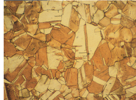
Pure copper. Sample etched with cupric chloride and ammonia. Magnification 100x. Sample
