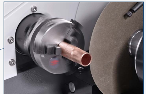
Rotation/oscillation reduces cutting time and avoids overheating of hard materials
