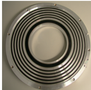
Fig 6: Rotating inductive transmitters at Ro 130
