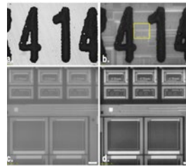
a. Brightfield image 5x, b. IR image 5x (BP1100 nm filter), c. Cropped detail 20x, d. Cropped detail 20x IR with DCE filtering
