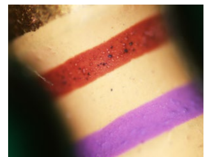
Composite image of several images with directional darkfield from different angles.
